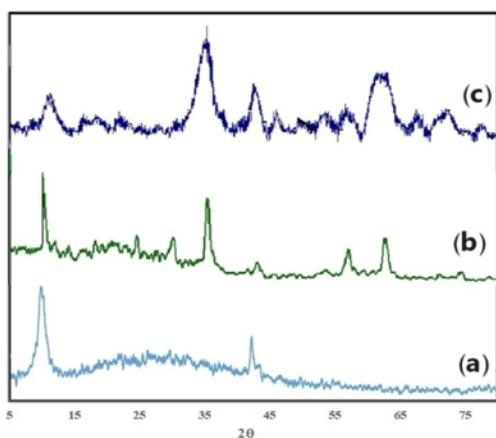
**Fig. 2.** XRD patterns of a) GO, b) MGO and c) MGO-IDA
