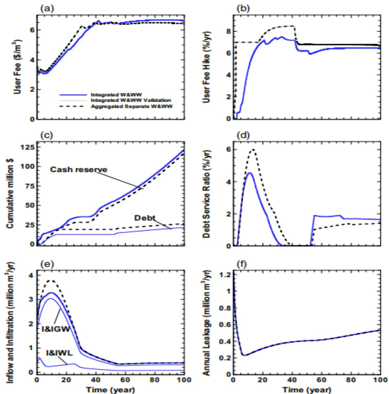
Fig. 6. Results over a 100-year simulation period (water and wastewater)
