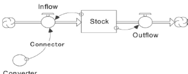
Fig. 2. Building blocks of system dynamics model
