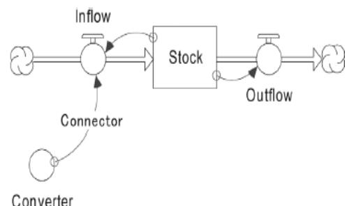
**Fig. 1.** Building blocks of system dynamics model
