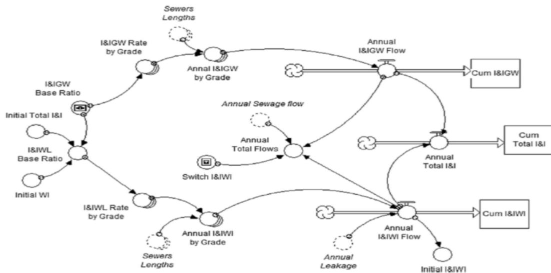
**Fig. 3.** I&I calculations for the integrated infrastructure sector
